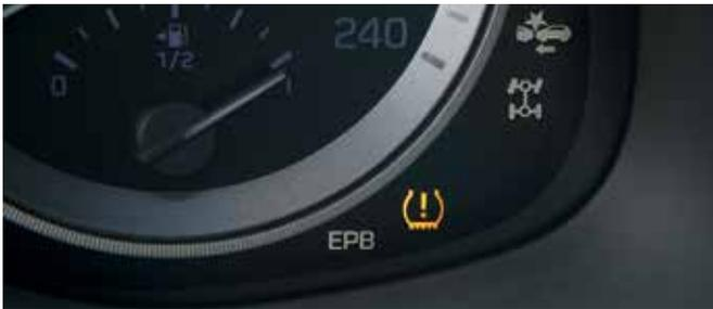
If your vehicle is a 2008 or newer (and some earlier models), it has a Tire Pressure Monitoring System (TPMS). It is designed to do exactly what its name suggests – keep tabs on tire pressure and alert the driver if the pressure in one or more tires falls more than 25 percent below the manufacturer's recommendations.
